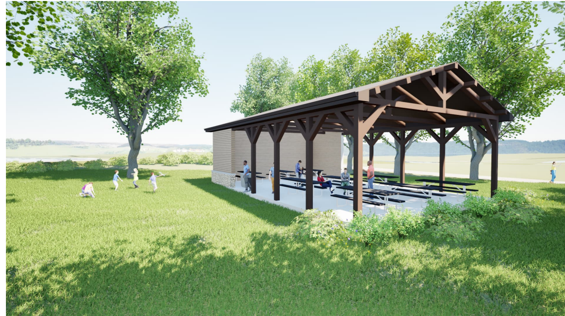
OPTION 2 - WOOD CONSTRUCTION - NO PONY WALL
