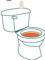
Return to the toilet where you placed colouring into the tank. Check the bowl of the toilet: is the water in the bowl clear or is there colour from the dye? If there is colour, water from the toilet tank is leaking into the toilet bowl. If the leak is large, you will be able to hear the toilet "running" and the dye will show up in the bowl
