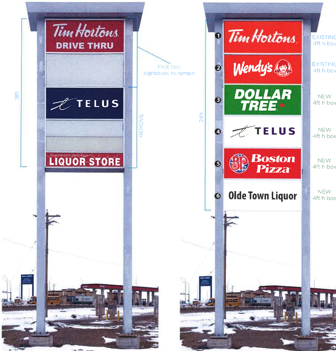
1-7 4-ft x 10-ft double-sided anodized silver sign boxes with acrylic inserts (and vinyl graphics as shown); internally illuminated with white LEDs
